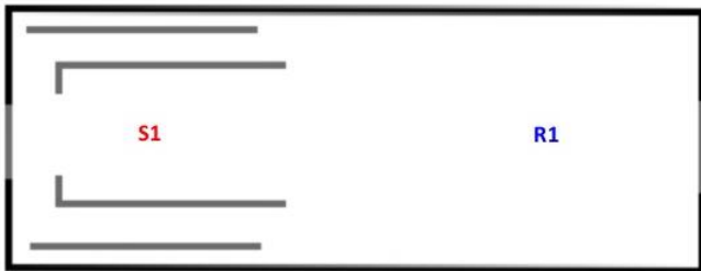
Figure 6 – Measured position in Divinity School, University of Oxford, dimensions: 27.6m x 10.3m x 7m, Volume: without furnishing 1989.9m 3
