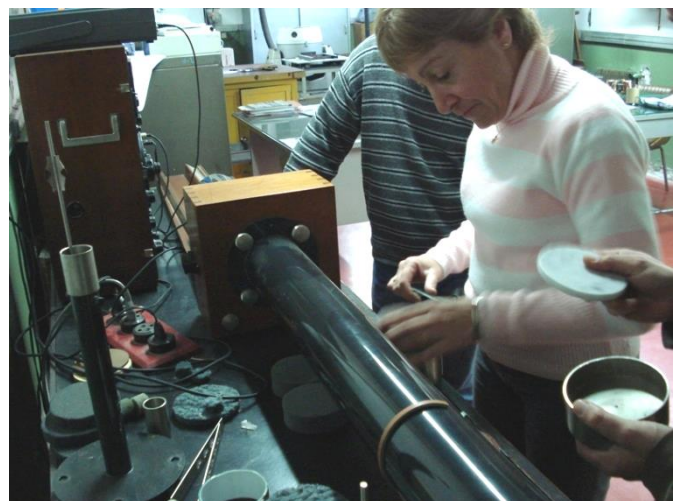
Figure 5 – Kundt tube measurement of the carpets for the Paradiso level
