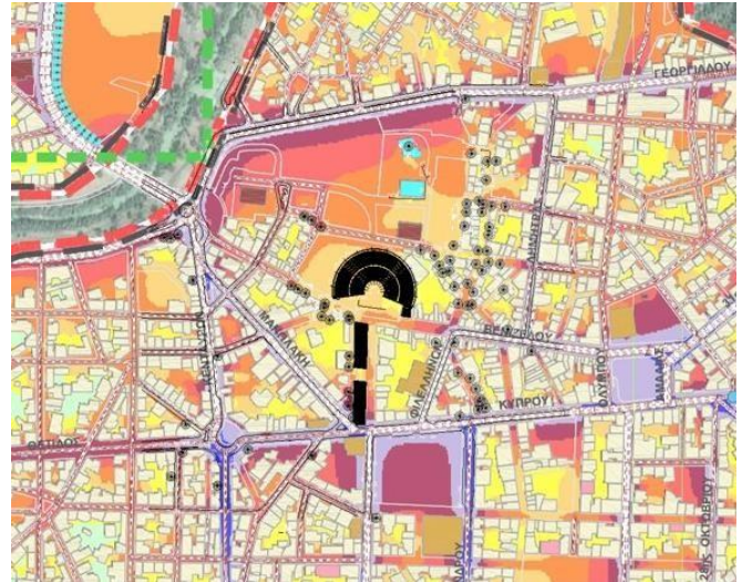
Figure 2 –Lden map with overlapping sound sources.
