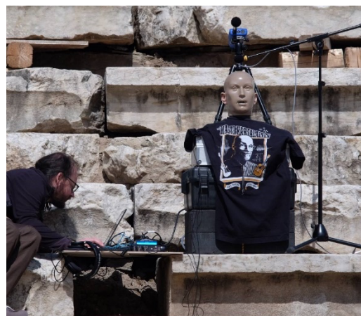
Figure 2 – Preparation of the measurement setup. It consists of the KEMAR binaural dummy head, the omnidirectional microphone and the SPL meter.
