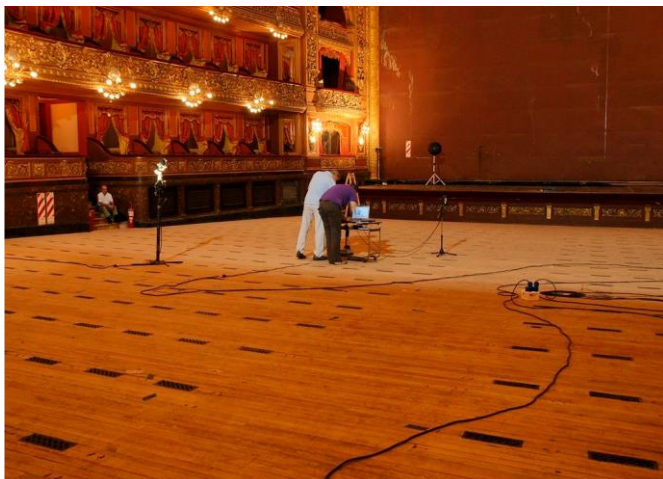
Figure 2 – Measurements in the hall after the removal of the stalls carpets
